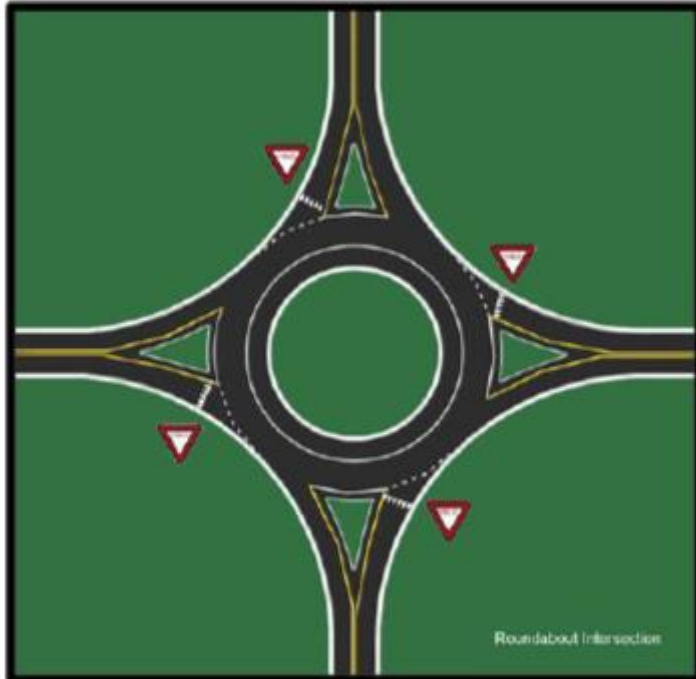
Figure 2-13: Sample Roundabout Intersection
